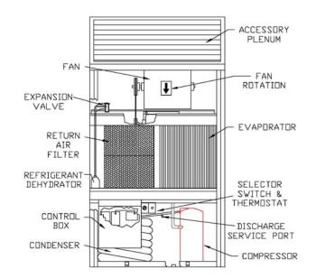
FIGURE 1 - BASE UNIT INTERIOR DETAILS (TYPICAL UNIT SHOWN)
